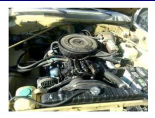
She has a 318 under her hood, a 3-speed automatic transmission with the column mounted shift lever, the original Chrysler solid-state radio in her dash with an Alpine AM/FM cassette under the AC vents (I intend to replace the Alpine with a unit that was contemporary in the '70s).
